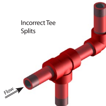
Figure 44 - Bull tee orientation "incorrect"
