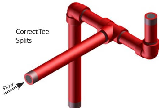
Figure 43 - Bull tee orientation "correct"
